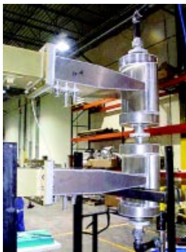
High-capacity (60-kW) cylindrical microwave heater with two consecutive in-line reactors, manufactured by Industrial Microwave Systems and installed in the CAPPS pilot plant at North Carolina State University
