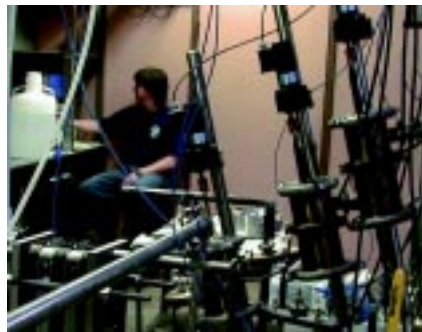
Research Associate Brian Heskitt operates the ohmic pilot plant at Ohio State University. The inclined objects are ohmic heaters
